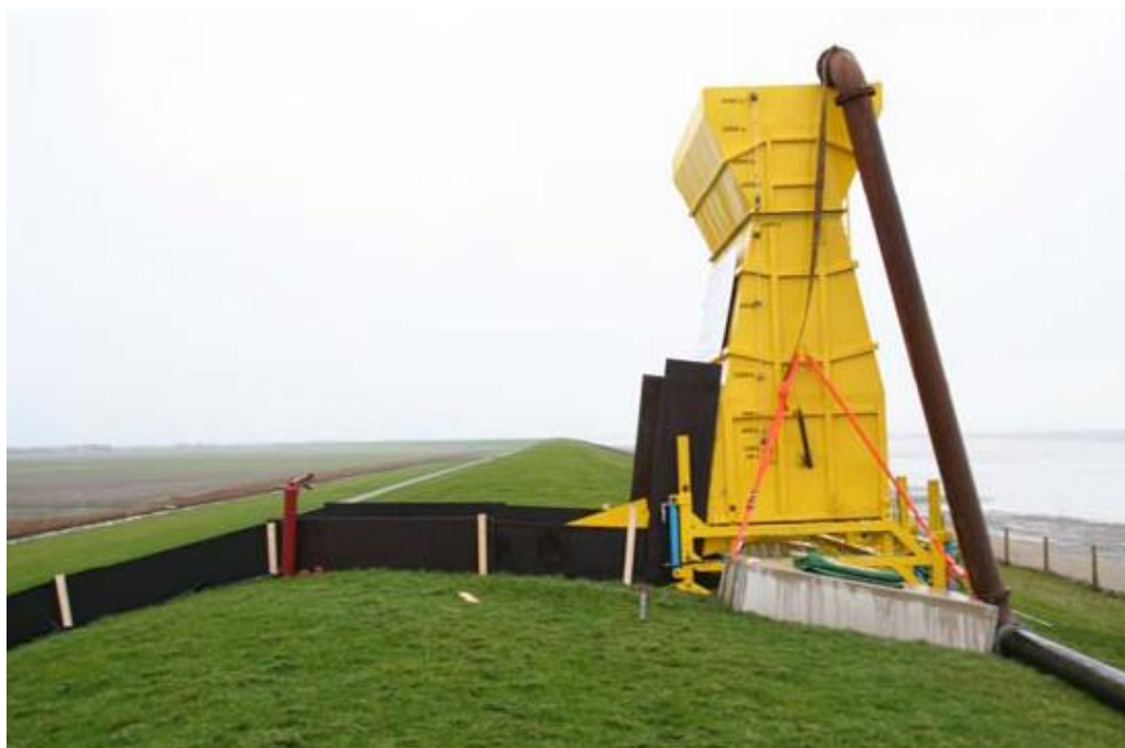
Figure 4-9: The wave overtopping simulator
