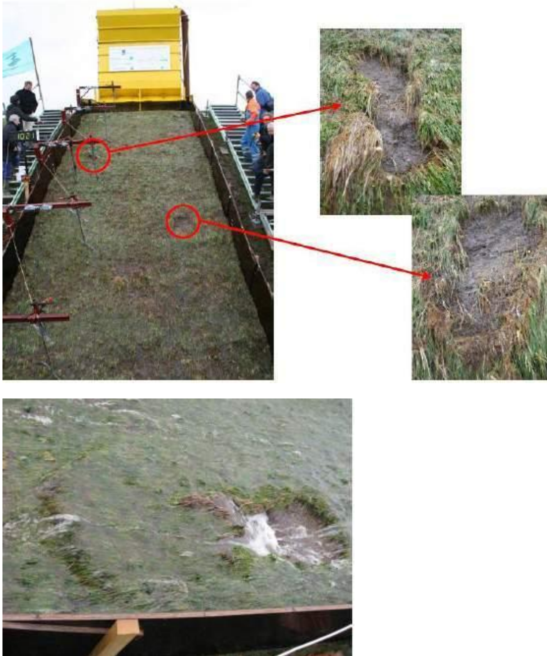
Figure 6-13: Example of initial damage; removal of small patches of grass sod (top) and a larger piece (bottom)
