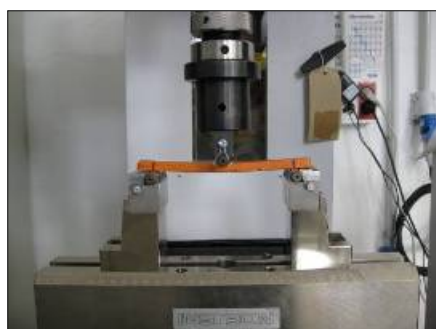
Figure 43 Flexural strength test - ASTM D 175.
