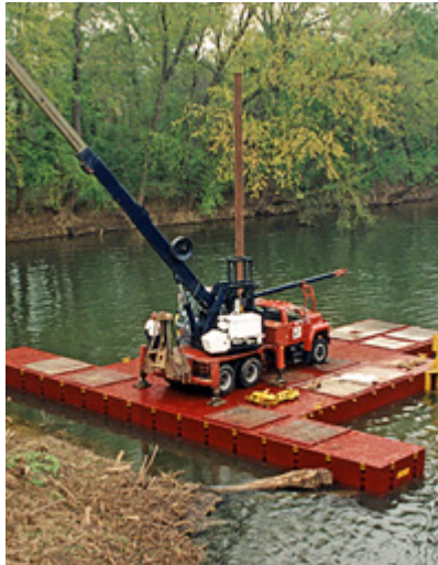
Figure 25 Example of box beam application, Flexifloat Inc.
