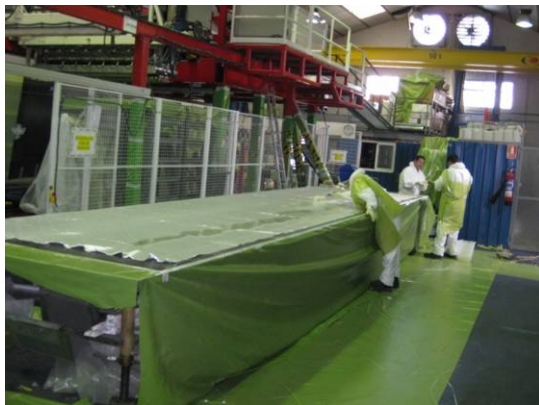
Figure 48 Glass fiber impregnation process.
