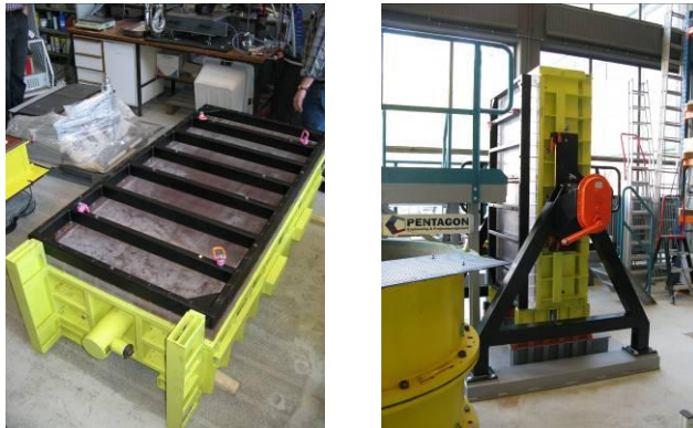
Figure 8 Medium scale experiment set-up BioGrout for backward erosion prevention
