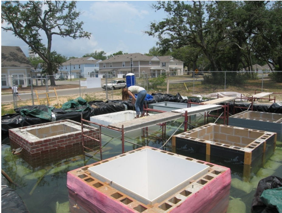
Figure 3.4 Tests of dry proof wall constructions at Oak Ridge National Laboratory, USA (from SERRI project, www.gccds.org )
